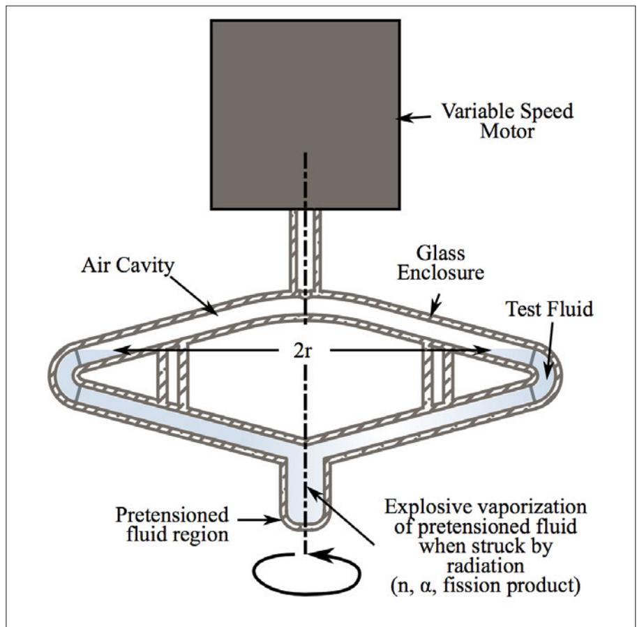
*Continued* **Fig. 2:** Schematic diagram of a centrifugally tensioned TMFD.
